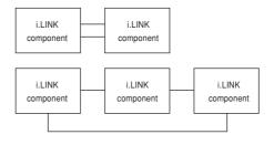
Do not connect devices in a loop as shown in the figure.
